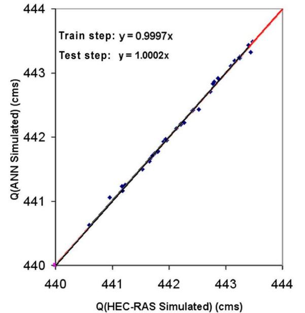
Figure 4. Scatter plot of maximum flood rate estimated by HEC-RAS model versus ANN predictions
