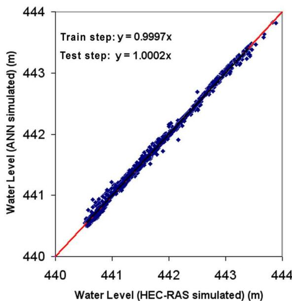
Figure 3. Scatter plot of maximum water level estimated by HEC-RAS model versus ANN predictions
